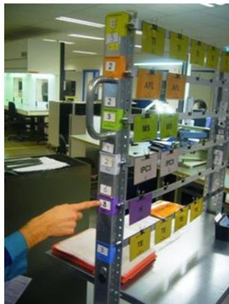
Figure 4. POLCA cards indicating the need for jobs. The manager points to the number of workers in a cell.
